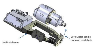
The motor controller frame attaches to the uni-body frame with a set of M8 socket head cap screws. The frame is CNC machined, like the uni-body structure, however it is designed to be removed and replaced as needed as the design of the system matures.
