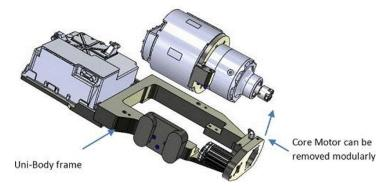
The motor controller frame attaches to the uni-body frame with a set of M8 socket head cap screws. The frame is CNC machined, like the uni-body structure, however it is designed to be removed and replaced as needed as the design of the system matures.
