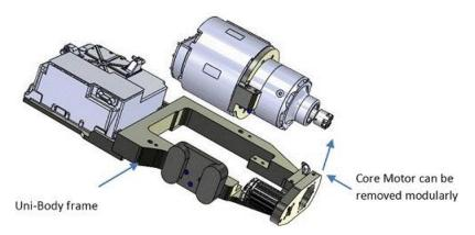
The motor controller frame attaches to the uni-body frame with a set of M8 socket head cap screws. The frame is CNC machined, like the uni-body structure, however it is designed to be removed and replaced as needed as the design of the system matures.
