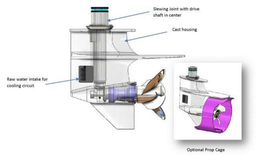
The propeller lower POD unit is expected to include a primary aluminum cast housing that is specifically engineered for electric propulsion. Because of the electric drive there is no need for the traditional reversing clutch mechanism or clutch actuation rod, or even the chambers for raw water exiting near the rear of the unit. This results in a lighter weight design with less parts and a more efficient drivetrain.
